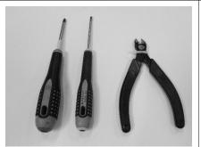
1. Use these tools to replace the lamp socket. A Phillips screwdriver, a flat screwdriver and a wire cutter
